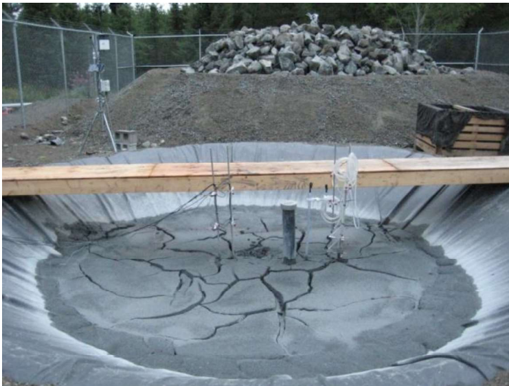
Figure 20-3: In-Situ Cells – Tailings cell in foreground, waste rock (serpentinized dunite) in background diameter of tailings cells is 5 m
